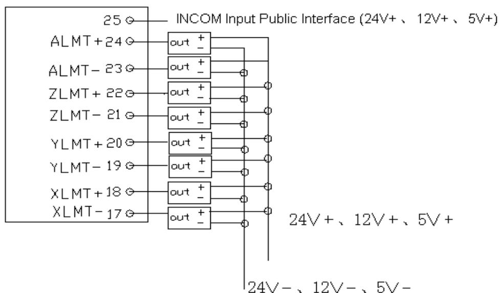
+Terminal is for the anode of power supply of the approaching switch, -Terminal is for the grounding wire of the approaching switch and the OUT terminal is for the output signal. For regular approaching switches, the operating voltage should be 10-30V, with NPN output. The photoelectric switch is also applicable.
