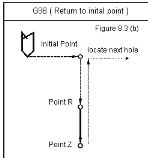
The parameters of hole to be machined are provided after G73/G74/G76/G81~G89, with format as follows:
