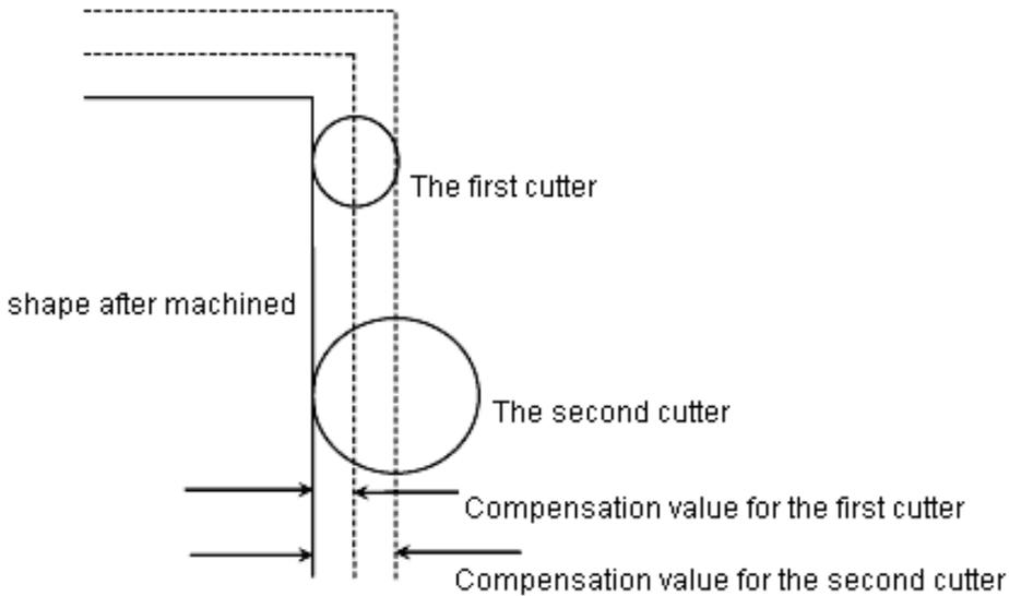
As shown in the following figure, the cutter with radius  $R$  is used to cut the workpiece  $A$ , the central path of cutter is  $B$ , the distance between path  $B$  and  $A$  is  $R$ . The process that the cutter leaves the workpiece  $A$  for some distance is called "compensation". Programmers use the radius compensation mode to produce the machining programs. In actual machining, the radius of cutter will be measured and entered into CNC. The cutter path becomes the compensation path  $B$ .
