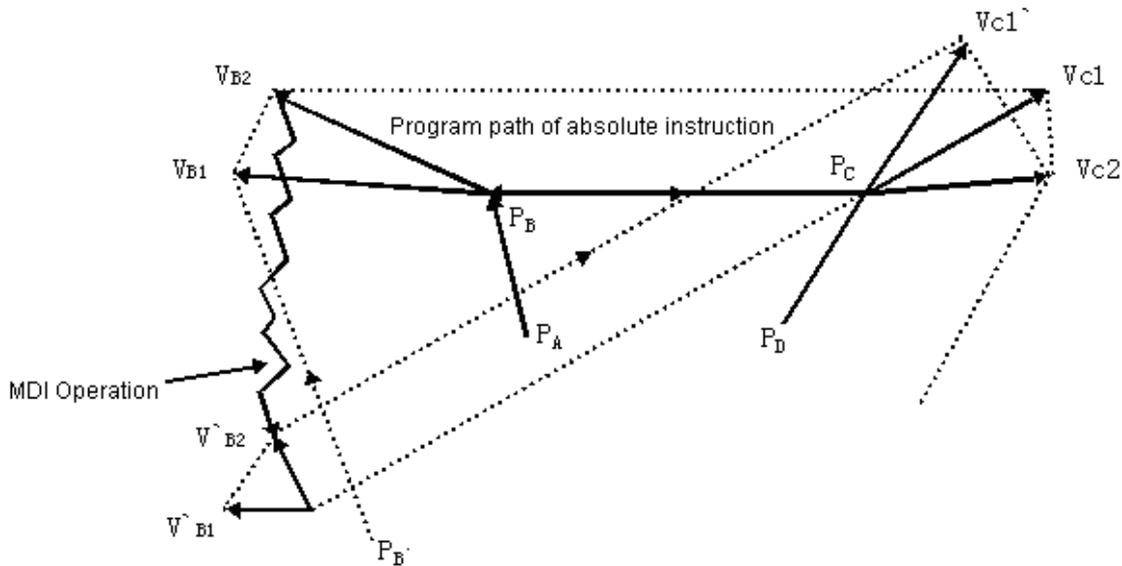
When point Pa, Pb and Pc are programmed with absolute instructions, the single segment will be used for stopping after the program segment is executed from Pa to Pb. The cutter is moved by inserting MDI. The vector Vb1 and Vb2 are transmitted to  $V_{b1}$  and  $V_{b2}$ , and the vector Vc1 and Vc2 between program segment Pb→Pc and Pc→Pd will be re-calculated.
