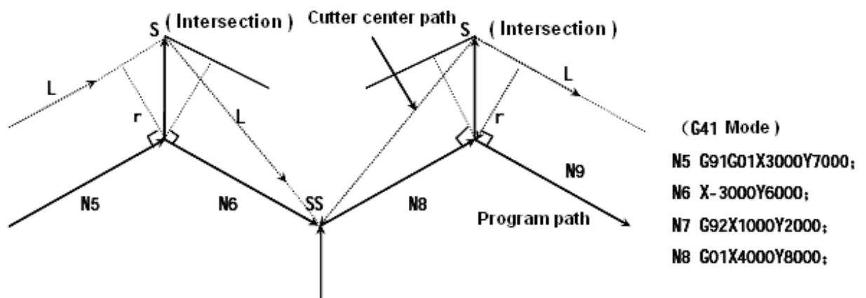
Note: SS indicates the point where the single segment mode cutter stops twice.
