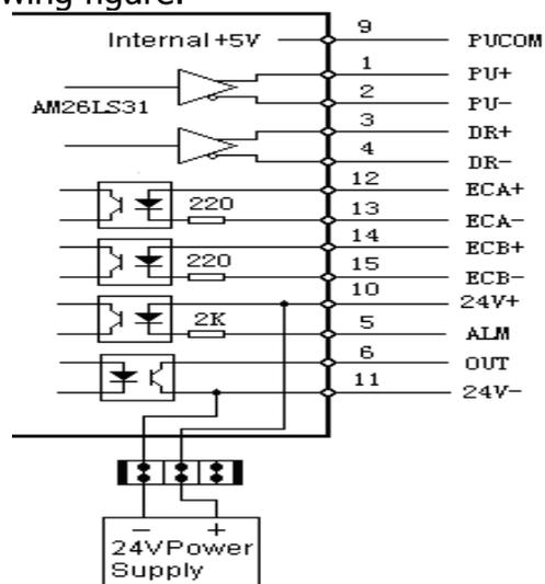
Internal Electric Diagram for Pulse Output.
