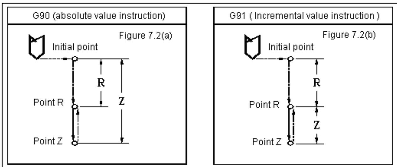
G98/G99 determines whether the cutter returns to point R or the initial point after the hole machining is finished in the fixed cycle. Under G98 mode status, axis Z will return to the initial point after hole machining. Under G99 mode status, it will return to point R.
