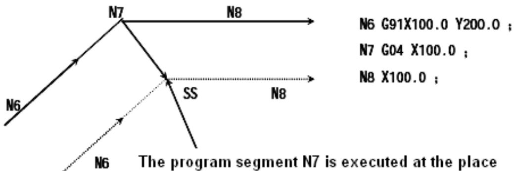
However, when the movement of the program segment is zero, even if only one program segment is designated, the cutter will move like the time there is no movement instruction. For details, please refer the following descriptions.
