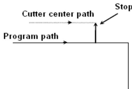
In left figure, the system will display the alarm information and the cutter will stop at the end point of the previous program segment .
