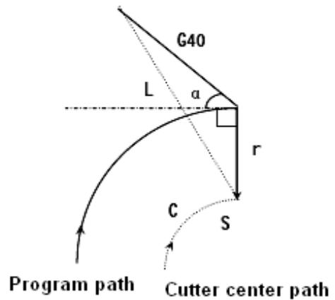
**(d) Move along the outer side of the corner which is an acuter angle less than  $1^\circ$  ( $\alpha < 1^\circ =$**
