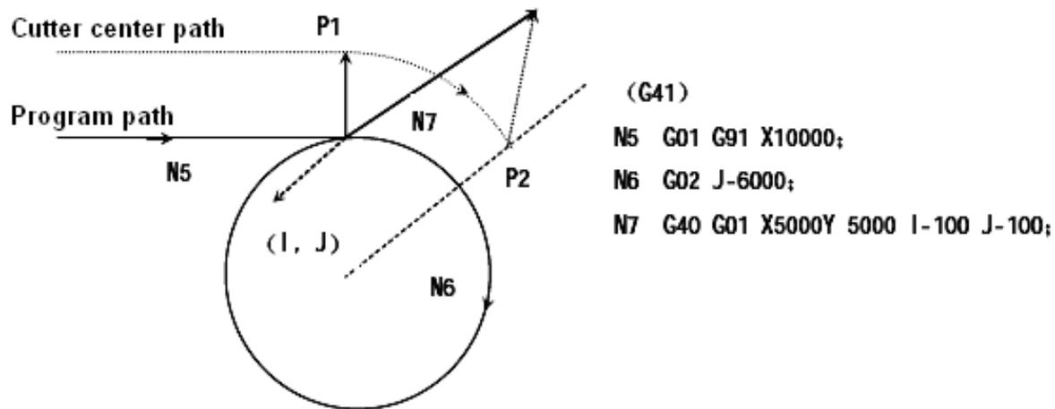
In above figure, the cutter center path doesn't move along the circle, but along the arc from P1 to P2.
