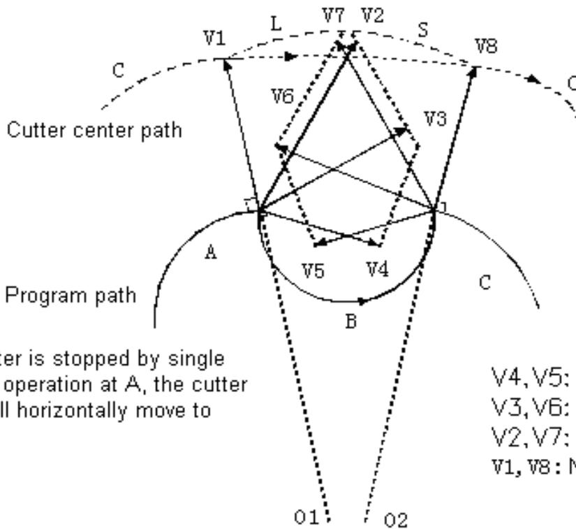
If the cutter is stopped by single segment operation at A, the cutter center will horizontally move to V3.
