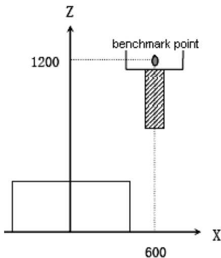
If some benchmark point on the hilt is considered as the start point, use the program start instruction G92. If the cutter moves according to the absolute value in the program, the cutter length must be compensated when it moves to the designated position. The compensation value is the difference between the benchmark point and the cutter tip.
