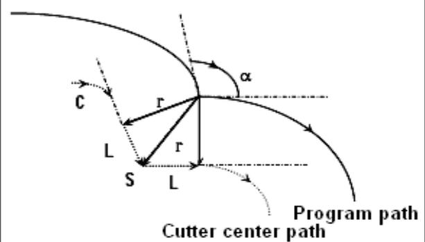
(c) Move along the outer sider of the corner which is an acute angle ( $\alpha < 90^\circ$ )
