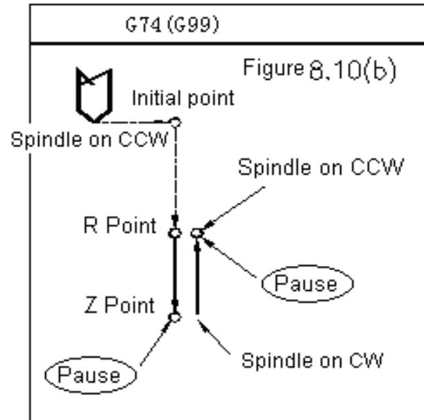
Notice: in the cycle of G74 and G84, the function of the feed rate switch and feed holding switch will be neglected, namely the feed rate will be keep at 100%, and it can not stop before a fixed cycle has been executed, the main shaft should be ordered to rotate around the tapping direction before the cycle.
