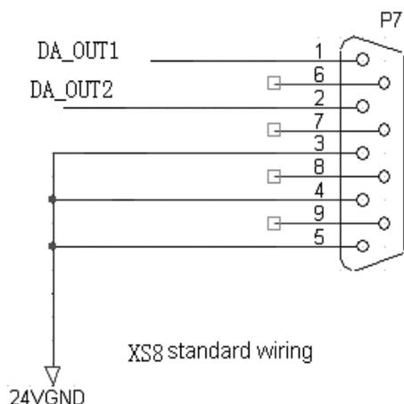
The standard wirings is suitable for XS8 interface of CNC4340,CNC4240 and CNC4342 controller.
