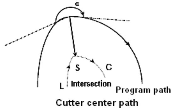
(v) Machining for inner side of less than  $1^\circ$  and compensation vector amplifying.
