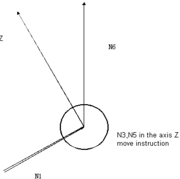
If the selected plane doesn't include the two program segments with movement instruction, N6 can't enter the buffering area, and the cutter center path will be calculated by N1, as shown in above drawing. If the compensation vector is not calculated at compensation start, over-cutting will consequently occur. Thus the abovementioned example must be modified as follows:
