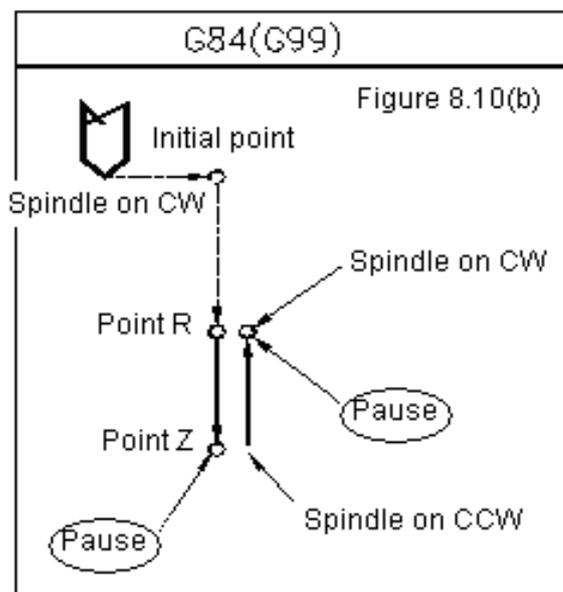
Notice: In the cycle of G74, G84, the function of feed rate switch and feed holding switch will be ignored, namely feed rate is kept at 100%, it can not stop before a fixed cycle is finished, you should command main shaft to rotate along the tapping direction before the cycle.
