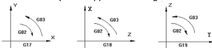
The end point of the arc is determined by the address X, Y and Z. In G90 mode status, which is the absolute mode status, the address X, Y and Z tell the coordinate value of the arc's end point in the current coordinate system. In G91 mode status, which is the incremental mode status, what X, Y and Z tell are the distances between the current point of the cutter and the end point along the coordinate axes.
