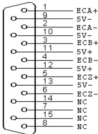
The standard wiring diagram of Spindle encoder:
