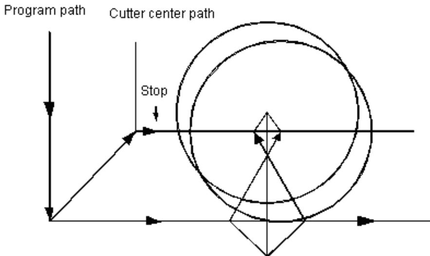
Like the example (1), the direction of cutter path is opposite to that of program path
