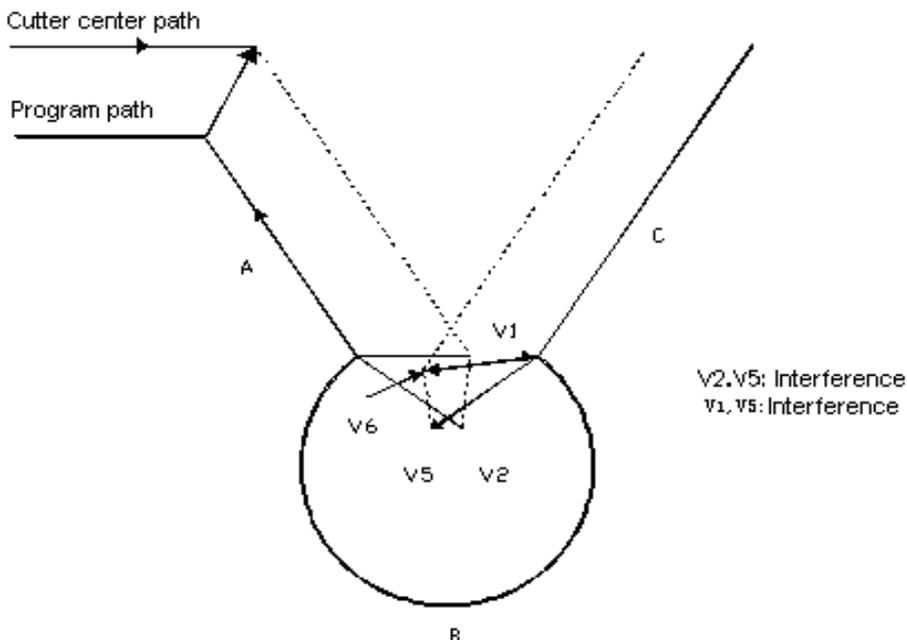
The interference ignores the vector V2 and V5. But interference will happen between the vector V1 and V6. The alarm information will be displayed and cutter stopped immediately.
