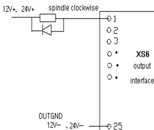
**Wiring diagram of machine(right)(take spindle on CW)**
