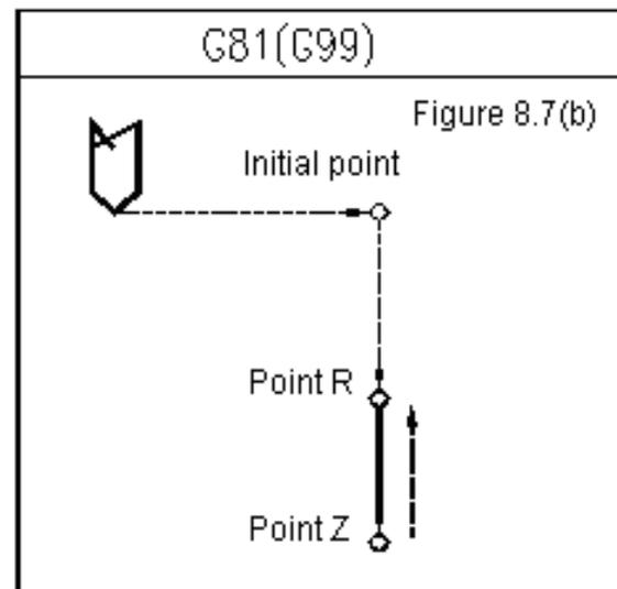
G81 is the simplest fixed cycle, whose execution process can be described as: after X, Y locating, axis Z fast moves to R, and moves to Z with F rate, then fast returns to initial point (G98) or R (G99). There is no action at the hole bottom.
