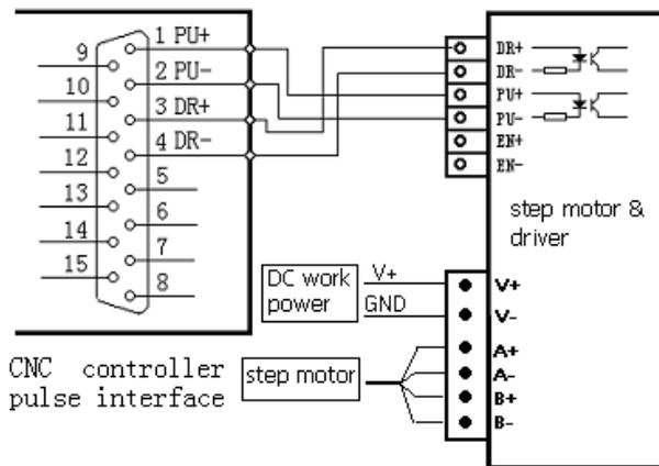
➤ Wiring Diagram to the driver of stepper motor with single-end input
