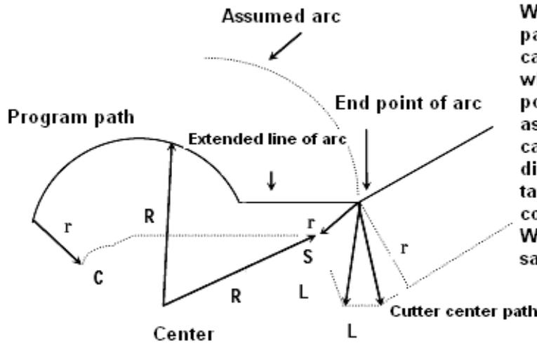
When the programming arc doesn't pass the end point, an extended line can be shown as in the left figure, which assumes an arc passes its end point. The compensation takes the assumed arc as its vector. In this case, the formed cutter center path is different from the offset path that takes the extended line into consideration. When it moves from arc-arc, the same consideration can be taken.
