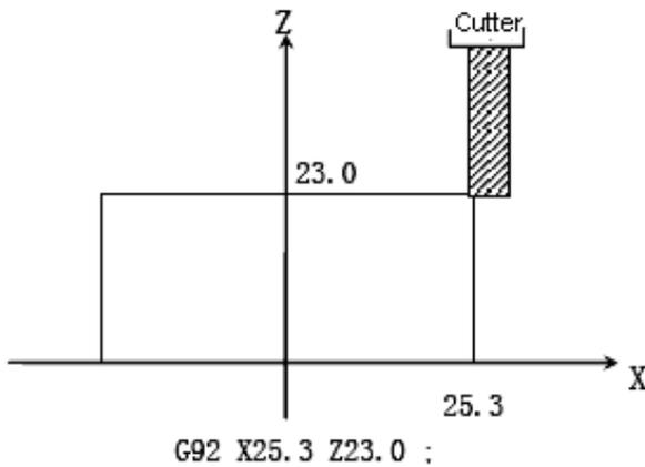
As shown in the figure, if the cutter tip is considered as the start point of the program, use the program start instruction G92.
