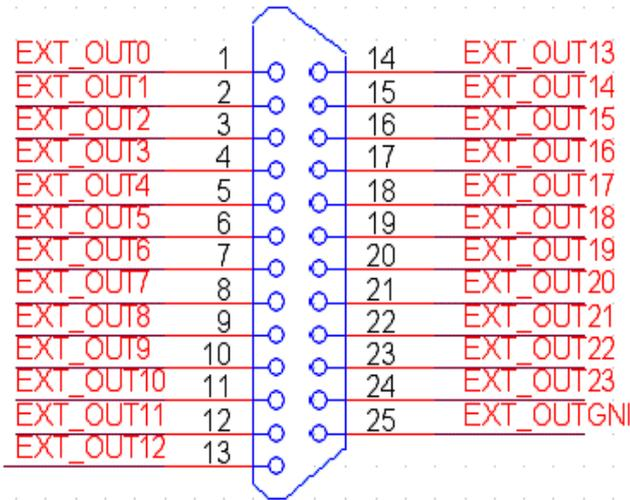
XS6 Output Interface Wiring Diagram
